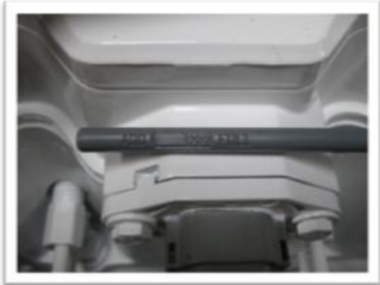
Figure 2 Newer engines have composite or high temperature plastic dipsticks.
