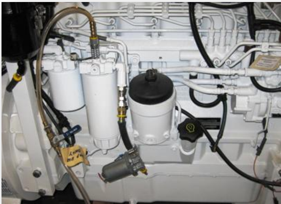
Figure 4 Next, plumb the electric fuel pump in-line with the incoming fuel to the primary filter as shown.
