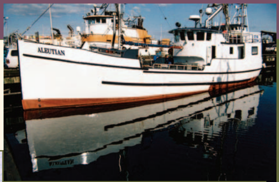
Aleutian —a 1928 wood displacement hull with 68'9" keel, 19'6" beam, 9' draft—enjoys greater fuel efficiency at faster speeds with a DEERE.
