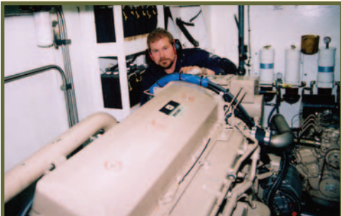
Engineer Todd Hoppe & Aleutian's MER-made factory-issue brown DEERE 6125AFM rated for commercial use: 341 hp @ 1800 rpm.
